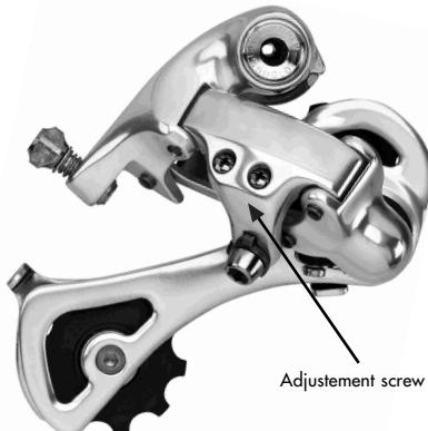
sprocket as possible but not so close that it touches. Next, set the chain to the smallest sprocket and repeat the above to make sure that the pulley does not touch the sprocket.
