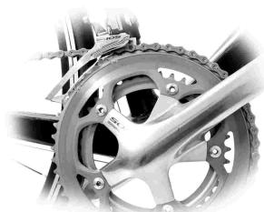
The derailleur should not protrude beyond the largest chain wheel by more than 2 mm and must not touch the pedal crank. For correct adjustment proceed as follows.
